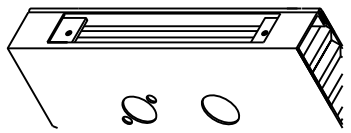
Closer reinforcement (if required)
